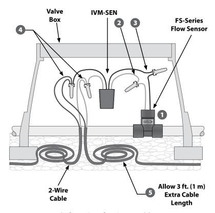
**Typical IVM-SEN Flow Sensor Wiring**
