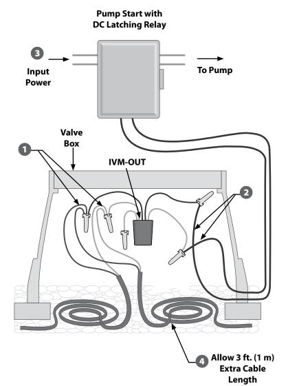
**Typical IVM-OUT Pump Start Relay Wiring**
