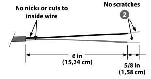
Remove the pre-cut insulation from the ends of the wires on the 2-Wire device. Connect the device wires to the 2-Wire path using linesman's pliers to twist the ends together.
